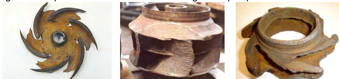
Fig. 17 Examples of Erosive Wear on Centrifugal Pump Impellers.
