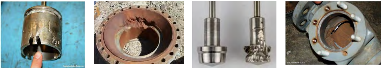
Fig.16-a Typical Erosion of some Control Valve Components in Contact with Slurries.
